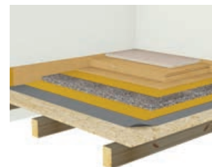
Wooden beam ceiling with AGEPAN® TEP
